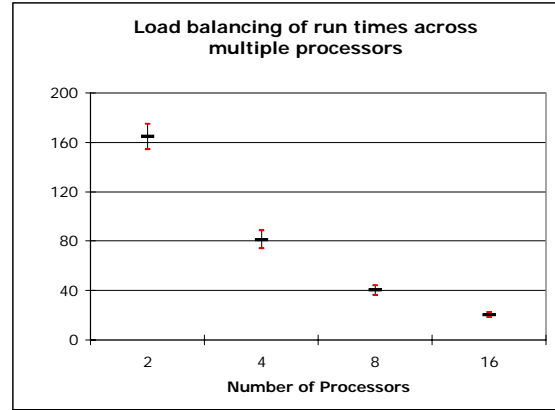
Figure 8. Load balancing of run times across multiple processors on the 2895 vertices graph with Init\_K=18 using up to 16 processors
