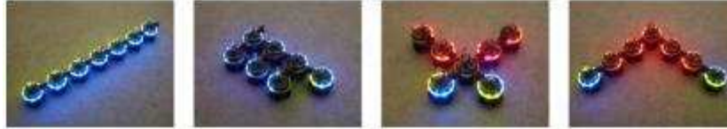
Figure 23. Structures generated from 7 real s-bots (line, rectangle, star, arrow) [26].
