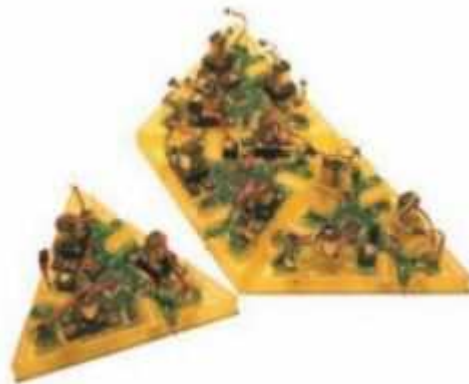
Figure 17. Programmable parts partially forming a triangle structure [2].
