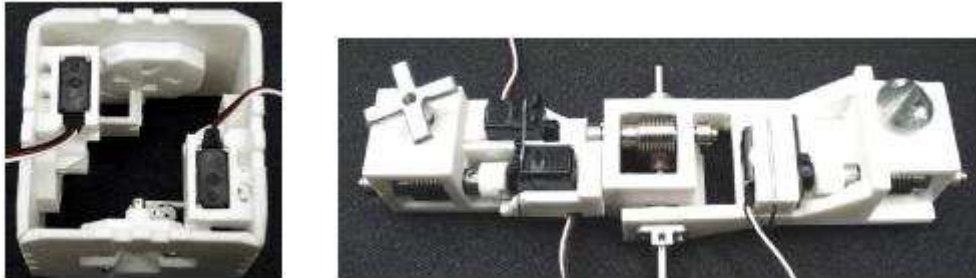
Figure 6. I-Cube cube structure (left) and link structure (right) [35].
