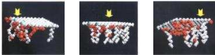
Figure 10. Table adjusting its legs according to position of weight [3].
