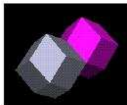
Figure 3. Rhombic dodecahedron shape of Proteo module [20].
