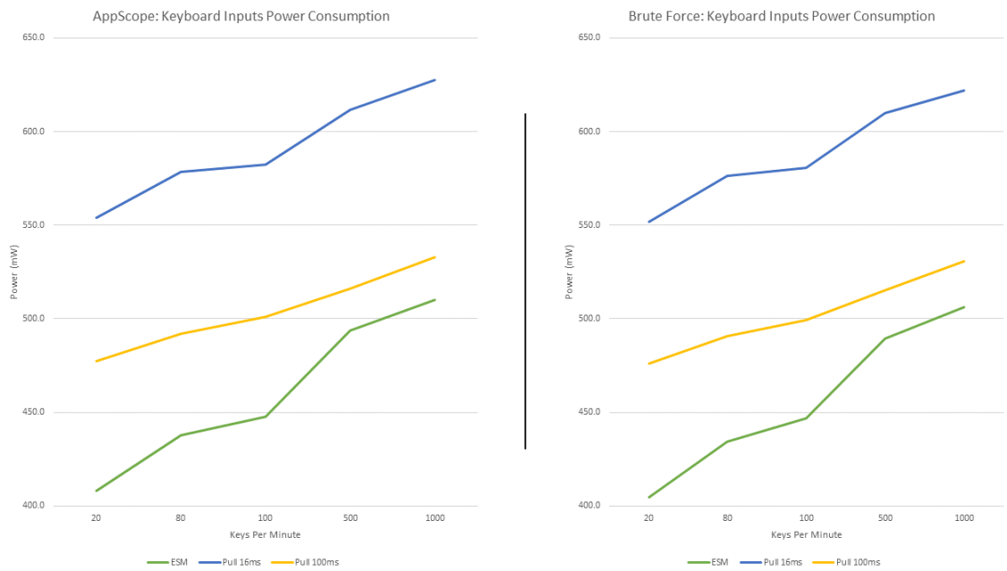
Figure 6.2: The keyboard inputs are by keys per minute. Roughly translated, 1000 keys per minute are 17 keys per second. This graph shows that the ESM model continually outperforms all pull models.
