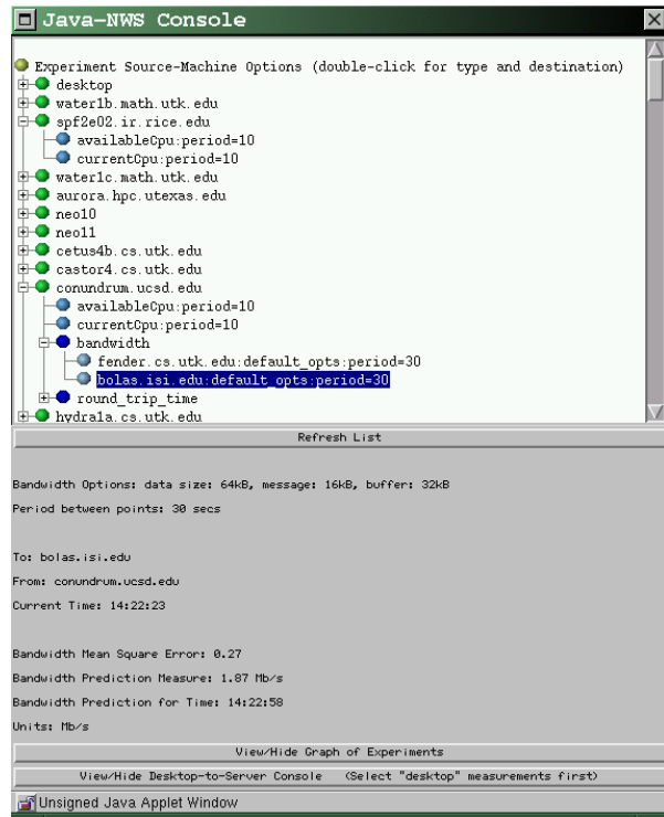
Figure 1: The NwsAlarm console. The console provides users with a click-able tree menu of machines for which NWS resource data is configured. The list can be refreshed to acquire dynamically added resources. For each machine, a list of resource types is given (network bandwidth and round-trip time, CPU availability and load, memory usage, etc). By selecting bandwidth or round-trip time, a list of the available destinations is given. In addition, network performance between the desktop and the server from which the NwsAlarm applet is downloaded is available for selection (“desktop”). The measurement data and predicted performance of the resource selected is displayed in graph form once selected.
